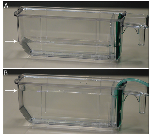
Figure 2. Larval tank assembly. A) The green baffle is inserted in the slot at the back of the tank. The 400 \mu\text{m} screen is inserted in the front-most slot, farthest from the green baffle. The tank is filled with \sim 250 mL medium so that the volume is level with the front angle of the tank (arrow). B) To refresh the tank medium, an additional volume ( \sim 400 mL) is added to the tank, raising the medium level as indicated by the arrow. To restore the starting tank volume, the siphon is inserted in the chamber between the screen and the baffle.
