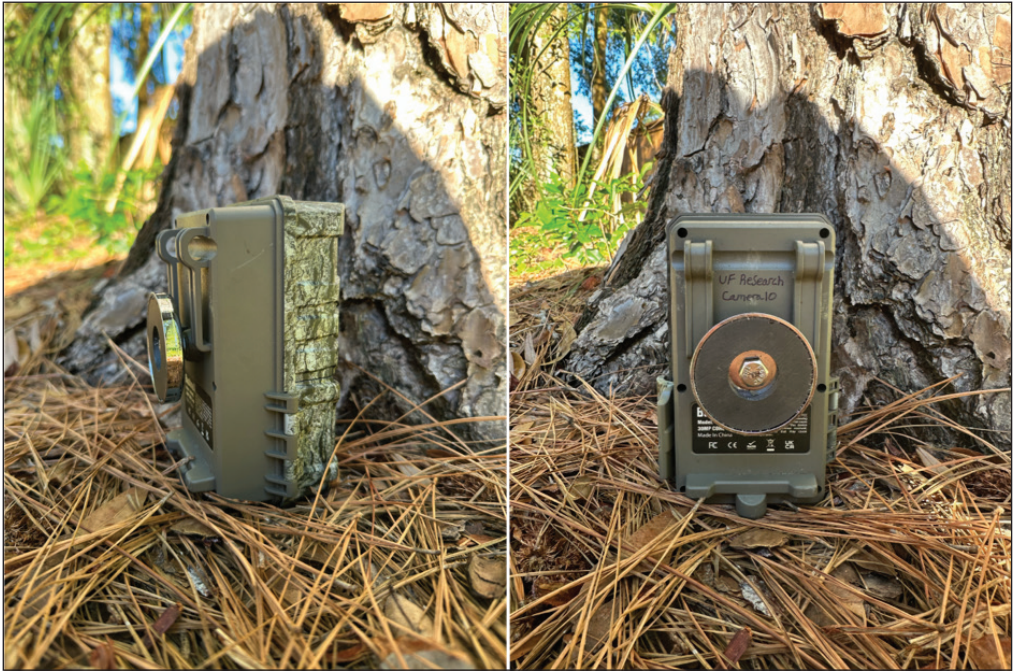
Figure 4. Example of camera-trap mount for magnetic attachment points such as manhole covers. Photo credit: Alan Ivory, UF/IFAS
